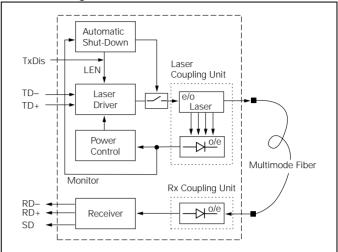
The receiver component converts the optical serial data into PECL compatible electrical data (RD+ and RD-). The Signal Detect (SD, active high) shows whether an optical signal is present.
